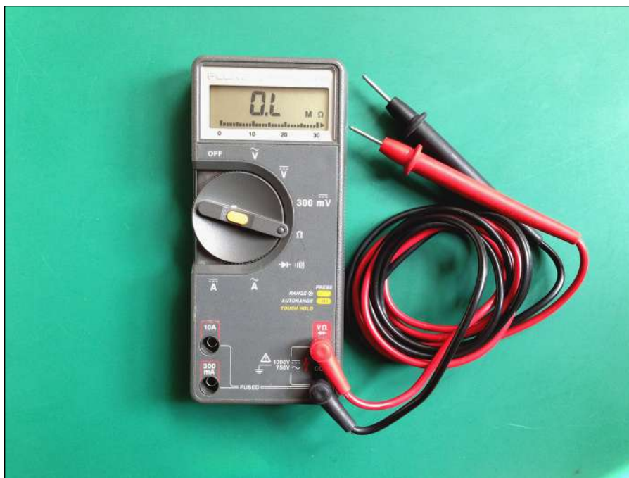
Figure 2-2: A digital multimeter is an essential diagnostic tool.
