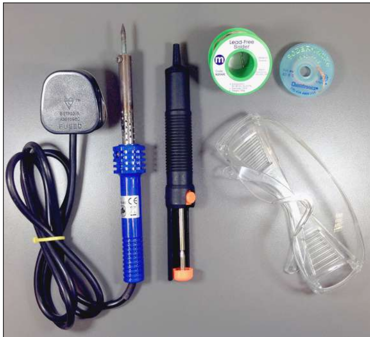
Figure 2-3: An entry-level soldering iron and essential accessories.
