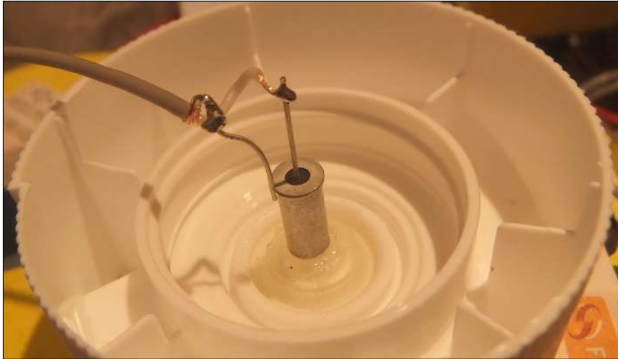
Figure 5-3: Wiring the screened cable to the tilt switch.
